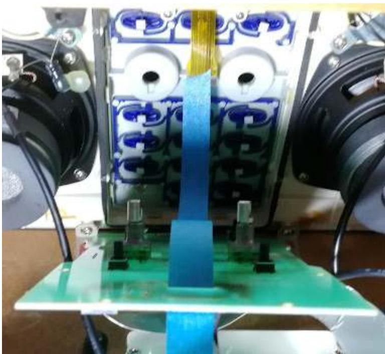
7. Connect the display cable. I used 2 toothpicks in the small holes of the display cable (see image) to move it up into position and then move the clamp up to secure it. Fold the small black cover back over the cable.
