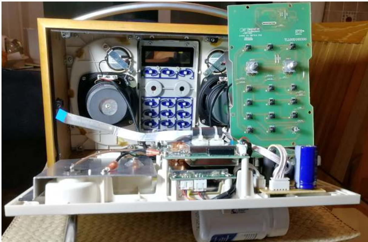
I chose not to remove the back panel but it would make it little easier to do so, but you would need to soldering iron for one of the wires. Suggest you put a cloth over the back panel components to prevent small screws or anything falling into it (I found out the hard way).
