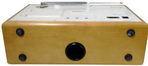
2. Remove the central black plastic cylinder from underneath the bottom panel. I removed the glue with a blunt chisel – it came away easily by twisting the chisel. Some of the glue was holding the front pcb in place. I removed that with a knife after removing everything else from the front pcb (next point).
