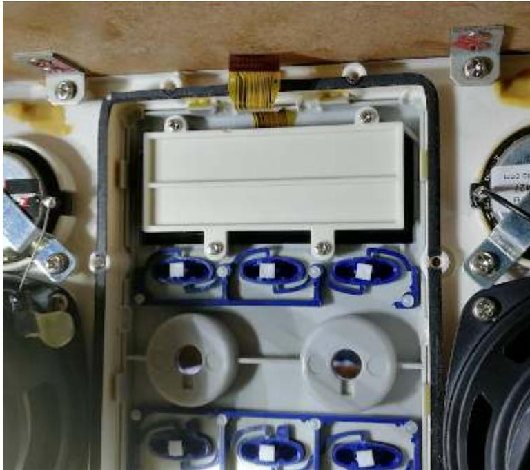
5. Refit the new display. Put the new display in the support with the cable coming out between the side that has the 2 screws with widest separation. This will ensure the cable comes out from the top (see image). Each screw hole in the supporting plastic panel has a recess that fits in the front panel so it can be positioned and held in place. Put in the 4 screws - into the side of the plastic support that is flat.
